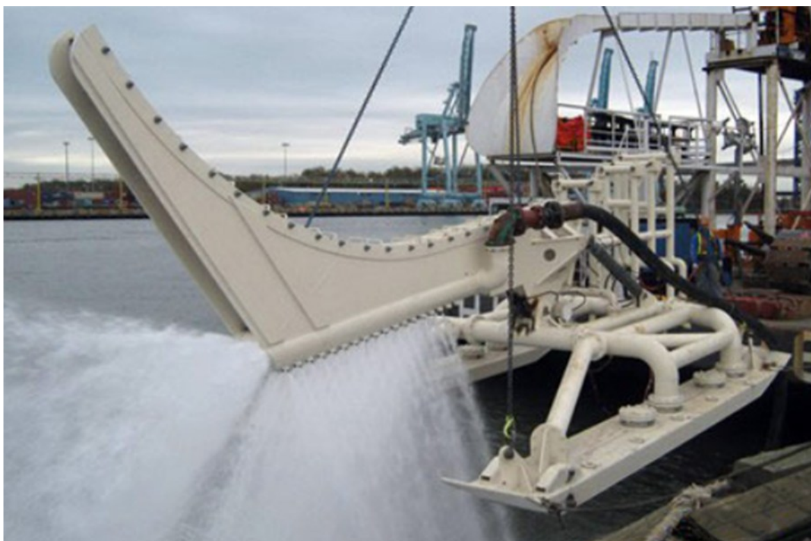
Figur 3.12 Mod-Jet/Sea Venture strømkabelslæde (kilde: https://eta-ltd.com/jetting-sleds-for-subsea-power-cable-laying/ )
